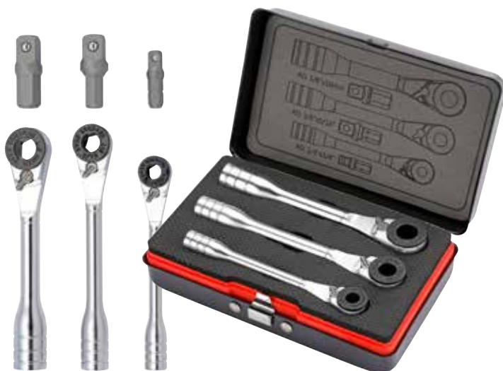
#100602 Mini ratchet set, 6-pcs This hand ratchet set contains three ratchets, suitable for 10mm bits, 5/16 bits and 1/4 bits. The ratchets can also be used for normal sockets with 1/2", 3/8" and 1/4" drive using the adapter supplied. This adapter can be stored in the handle of the ratchet.
