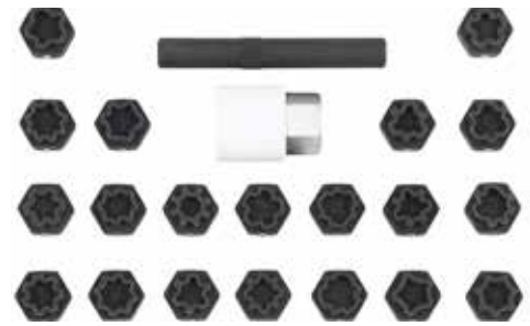
#829006 Wheel nut key set - Audi 22-pcs Audi set complete including 21mm adaptor with 1/2 "square drive. This kit is designed for the removal of locking bolts when the customer has forgotten to provide the adaptor with the car. This is happening very often when the vehicle is brought to maintenance and/or repair. Suitable for OEM T40073.
