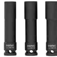
#300302 Torque impact adaptor set 1/2", 3-pcs - 17, 19, 21mm - Thin wall - plastic stop - 105mm - Maximum 200Nm
