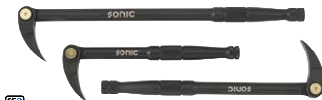
#805003 Universal ratcheting pry bar set 3-pcs For flexible use, for instance on bearings, belt pulleys, seals, wheel hubs, etc. The flexible heads on the pry bar can be fixated at 8 positions and safely locked via a pressure mechanism on the head end. The tapered head ends facilitate optimal use even with a minimal working gap. In the following lengths for each pry bar: 250mm, 300mm, 380mm.
