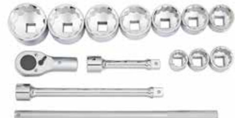
#501401 Socket set 1", 12 pt. 15-pcs - Bi-hex sockets: 36, 38, 41, 50, 55, 60, 65, 70, 75, 80mm - Extensions 200 - 400mm
