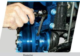
Universally suitable for ABS sensor mounting holes with a bore diameter of 18 mm.
